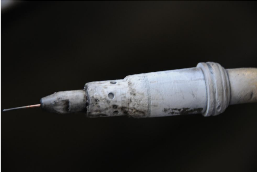
Welding torch coated with Weld-Max A
